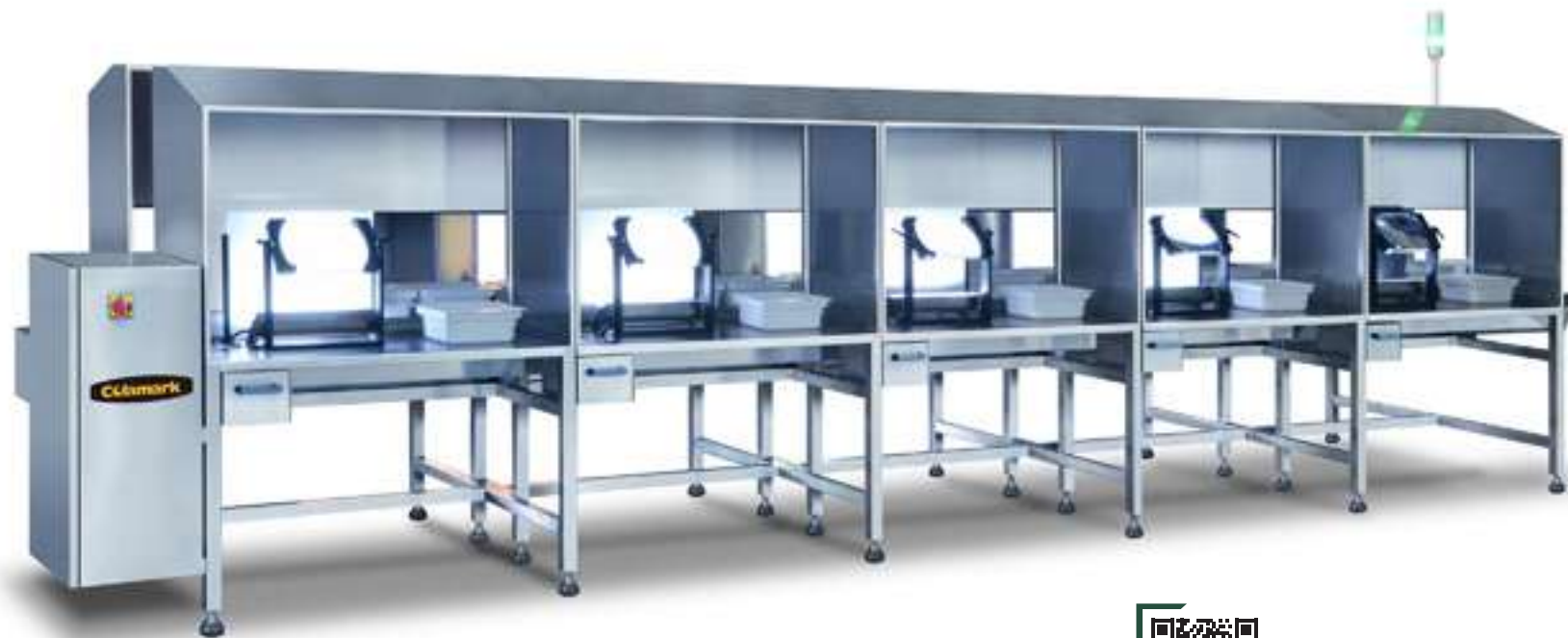
10-stations semi-automatic visual light inspection system
